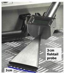
Scanning is performed with a suitable fishtail probe attached to the photometer inlet tubing. After setting the photometer as described in 6., the filter face should be scanned in overlapping scans approximately 30mm from the filter face at a rate derived from the formula in BS EN ISO 14644-3:2005 (B.6.2.5), which says that the scan rate should be approximately 15/Wp cm/s, where Wp is the probe dimension perpendicular to the scan direction. If the probe is 3 cm wide, the scan rate is 5 cm/s.
